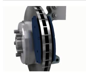
As the brakes are applied, a tiny amount of the friction material on the brake pads is worn off.
