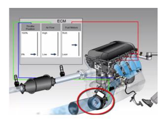
A hot wire system is preferred because it causes very little restriction to airflow, although it does become contaminated under prolonged use.
