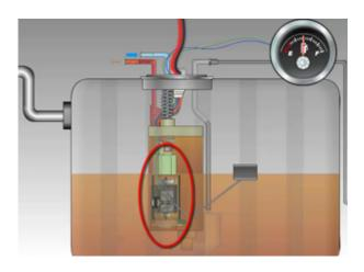
The fuel pump itself is submerged in fuel to aid in cooling.
