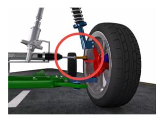
Tie rods push and pull the wheels in the designated direction.
