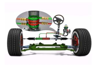
When the steering wheel turns, the rotary valve in the rack and pinion assembly opens to provide pressurized fluid to provide steering assistance.
