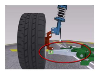
The lower control arm allows the wheel to move up and down, independent of the subframe.
