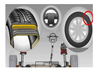
Tread separation refers to when tread pulls away from the steel layer of the tire, creating a bump in the surface of the tire.
