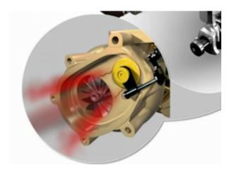
Over time, the wastegate seal can crack, allowing exhaust gases to escape and causing a loss of intake air pressure.
