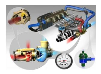
The turbocharger uses moving exhaust gases to compress air entering the intake.
